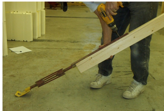
Figure 20: Photographs illustrating turnbuckle system.
